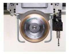
A manual coolant nozzle unit is our standard equipment for the Multigrind® CU.
